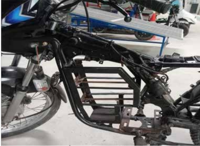
Figure 11.7: Conversion of Scrap Vehicle into Eco-Friendly Vehicle Battery Electrical Vehicle by Govt Model ITI, Hosur Road, Bengaluru.
